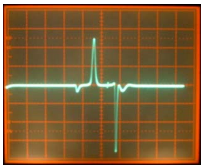
Typical Output Horizontal: 20ms/div Vertical: 100mV/div
