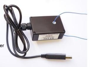
This interface is powered by the computer to which it is connected. Many phones and tablets can use an FTDI adaptor and be set to the AptiLoop speed of 1200b/s to monitor or adjust the AptiVolt modules included in the cluster—which can vary from 1 to 10.
